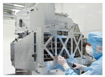
Vacuum chambers, which have to meet the highest standards in terms of dimensional accuracy and precision, are made from our ACP5080 S material. These chambers are machined in alimex's CNC department.
